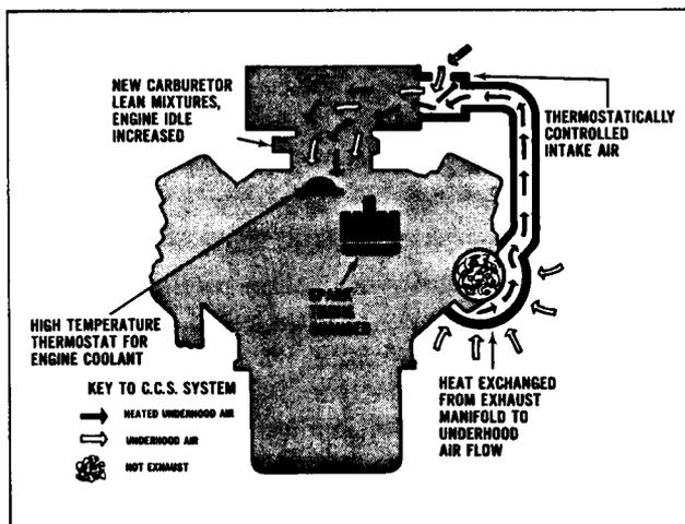
One method of controlling exhaust emissions involves the Controlled Combustion System (CCS) which is entirely separate from the Positive Crankcase Ventilation System. CCS is designed to reduce pollutants in the exhaust by improving the combustion process. It consists of a combination of design features including a special air cleaner which incorporates thermostatic control of heated air to the carburetor, a special calibrated carburetor and distributor and a modified combustion chamber design.
