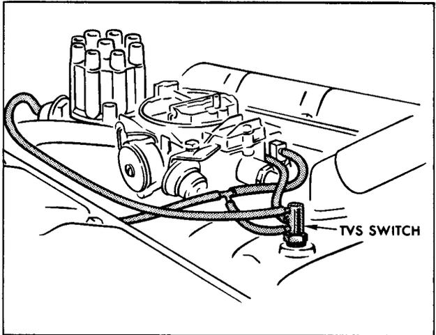
The retarded spark setting at idle speeds required for effective emission control makes engines tend to run hotter during idle or low speed conditions.
