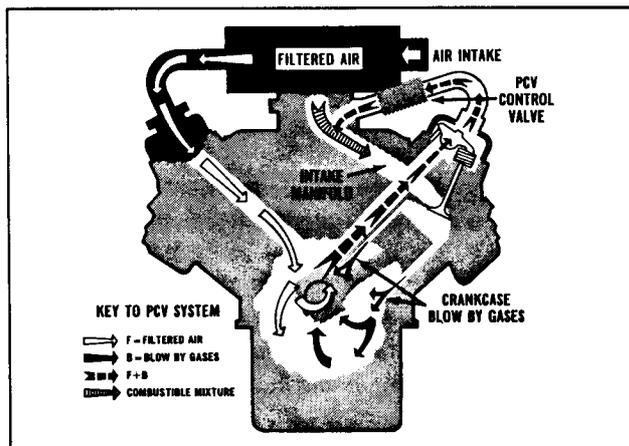
All General Motors gasoline engines are equipped with Positive Crankcase Ventilation — a system which permits no crankcase emission to be discharged into the atmosphere. To function properly, the system depends on the PCV Valve which returns blow-by gases to the combustion chambers where they are burned.
