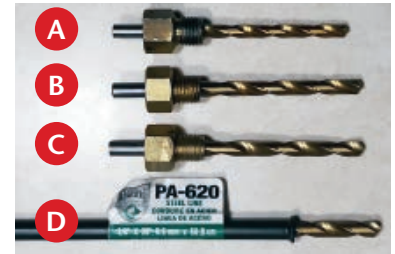
A. Original 5/16 line fitting with .244 hole B. 3/8 line fitting with .282 hole C. 3/8 line fitting with .312 hole D. 3/8 tubing with .312 ID
